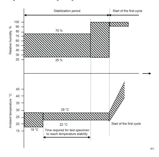
Figure 3 – Test – Recovery at controlled conditions
