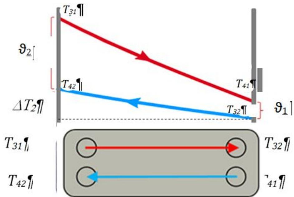
**Figure 3 — Variables in a DHW counter-flow heat exchanger**
