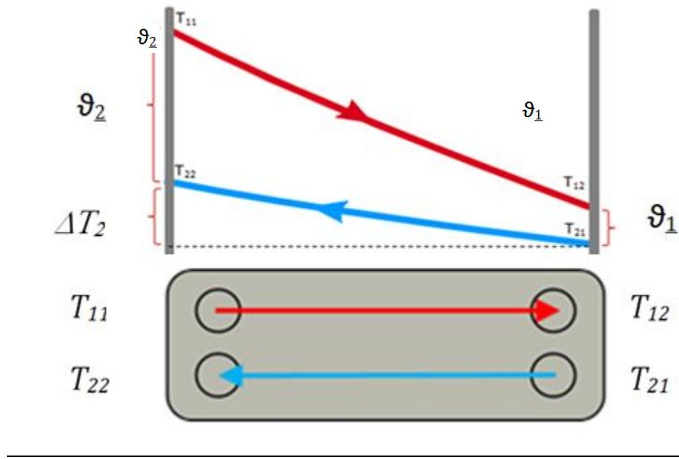
Figure 2—Variables in a heating counter-flow heat exchanger
