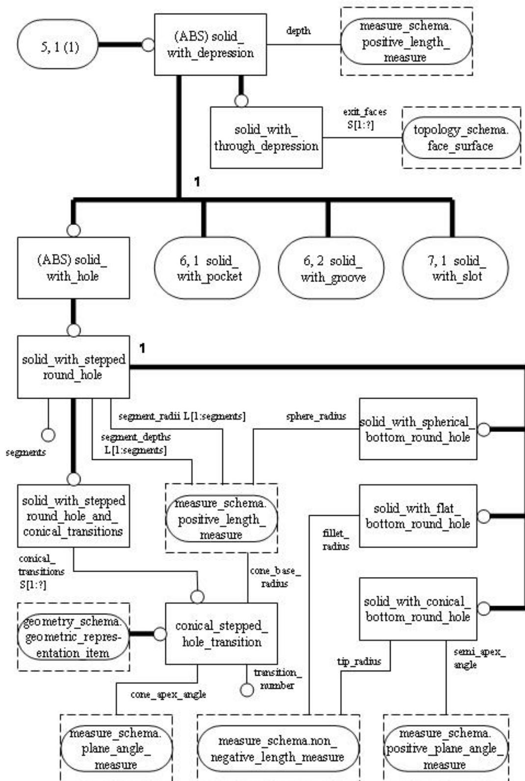
Figure D.5 – solid\_shape\_element\_schema – EXPRESS-G diagram 5 of 11
