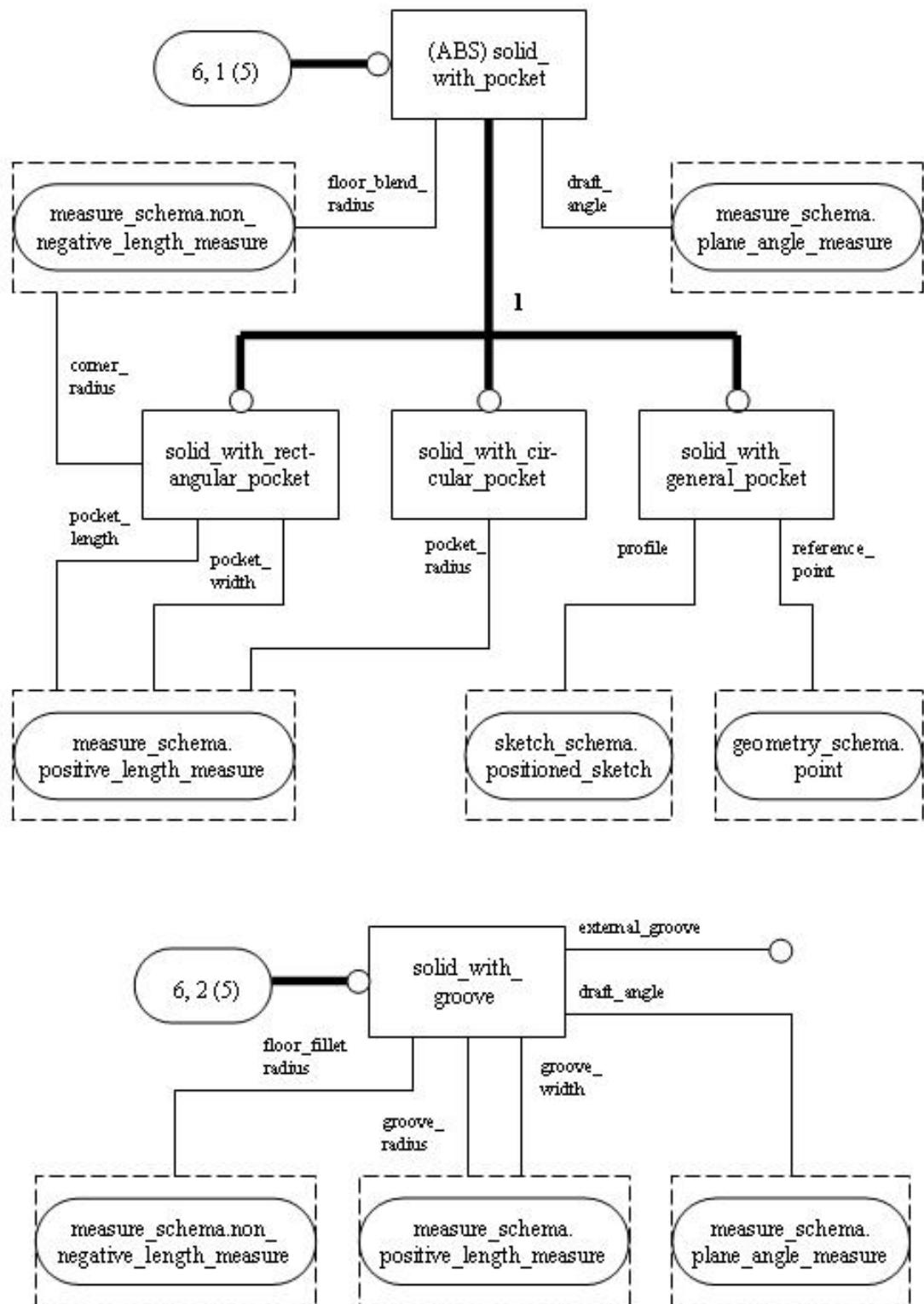
Figure D.6 – solid\_shape\_element\_schema – EXPRESS-G diagram 6 of 11
