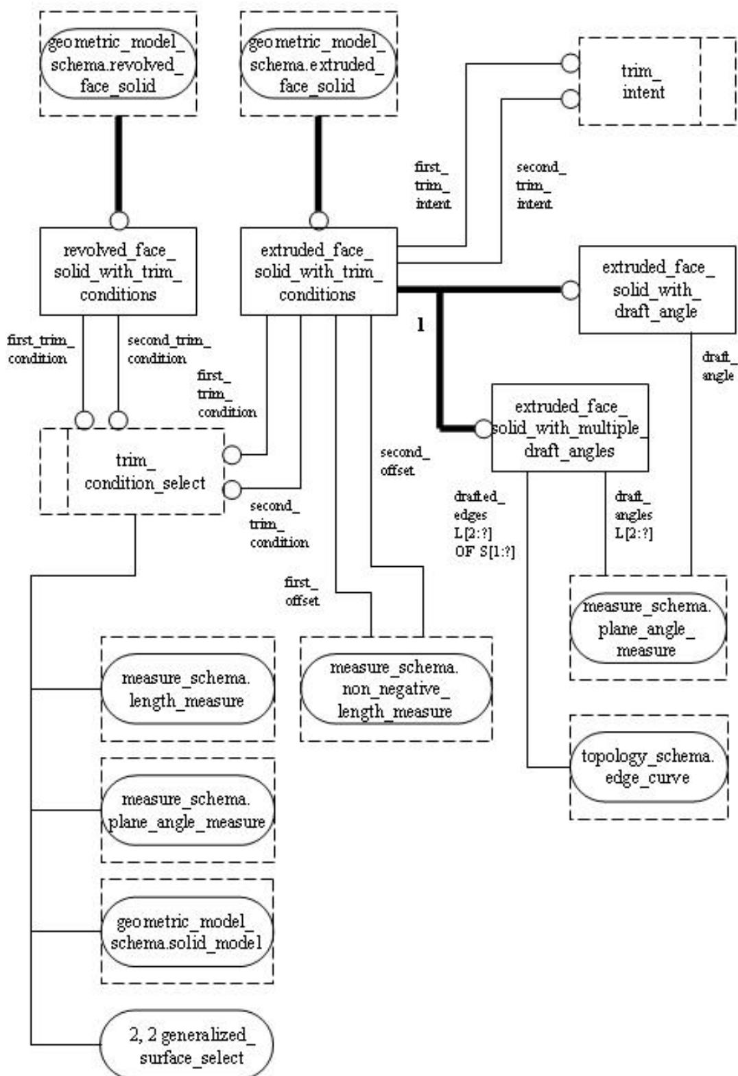
Figure D.10 – solid\_shape\_element\_schema – EXPRESS-G diagram 10 of
