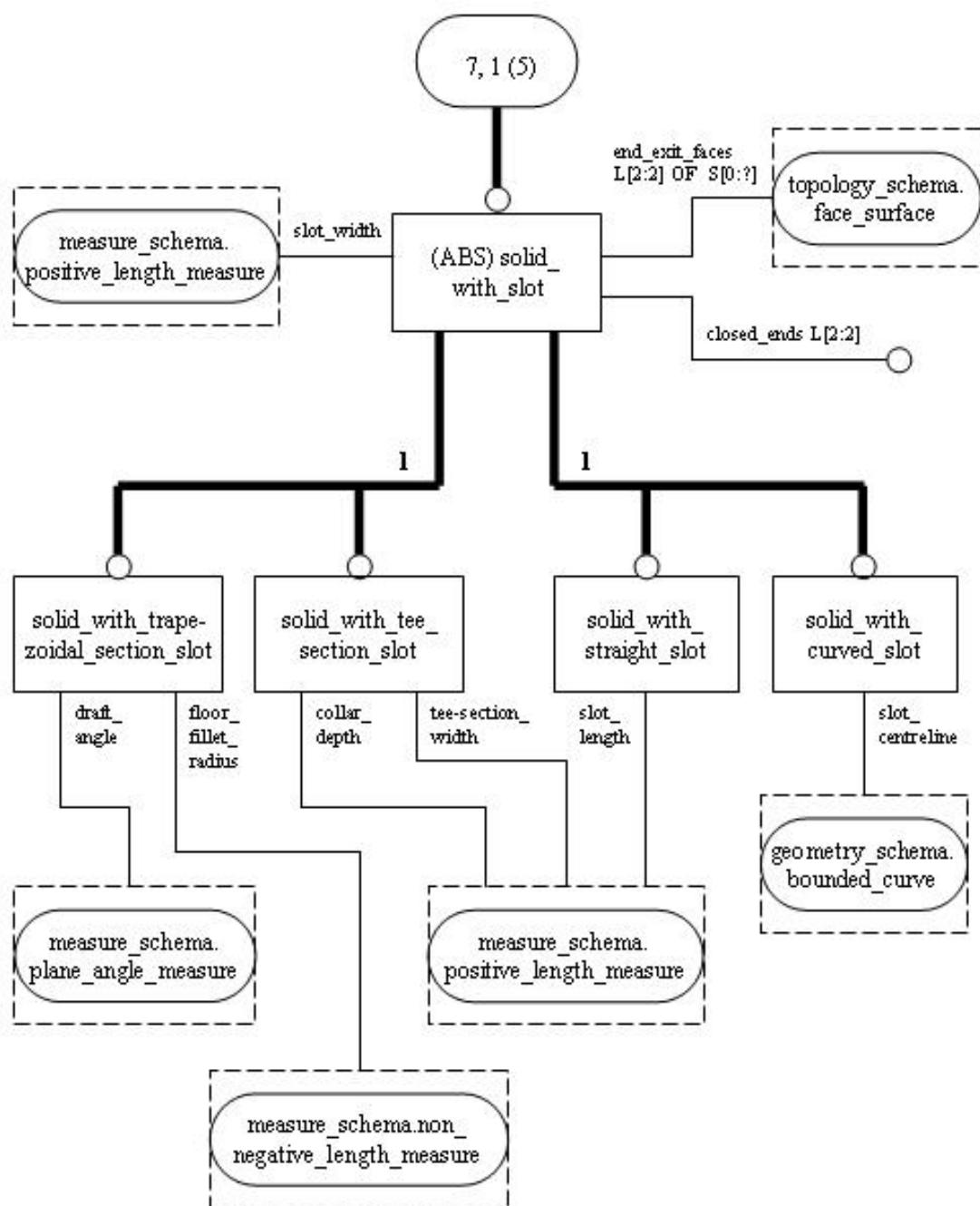
Figure D.7 – solid\_shape\_element\_schema – EXPRESS-G diagram 7 of 11
