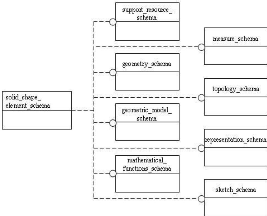
**Figure 1 – Schema level diagram of relationships between the solid\_shape\_element\_schema of this part of ISO 10303 and other resource schemas**
