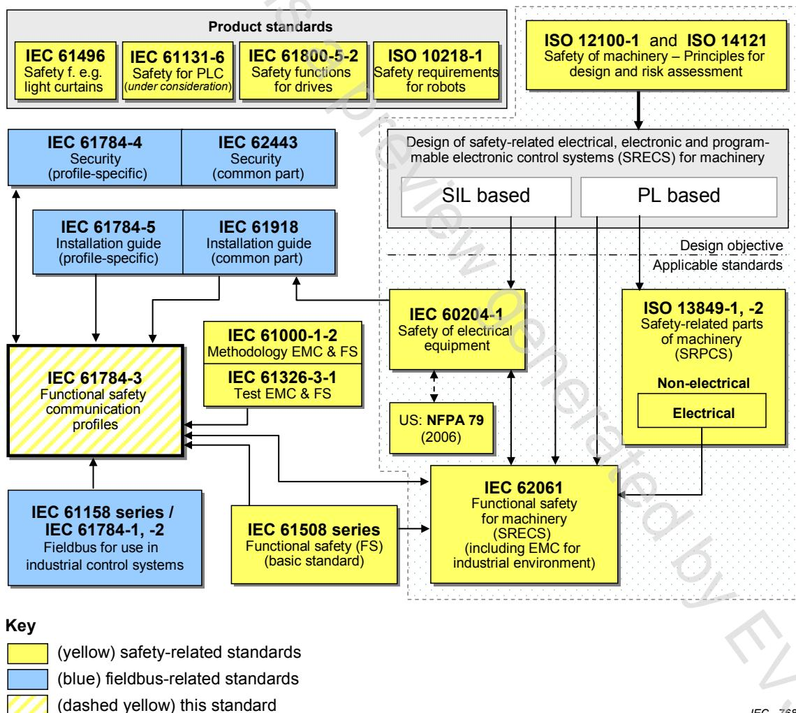
**Figure 1 – Relationships of IEC 61784-3 with other standards (machinery)**
