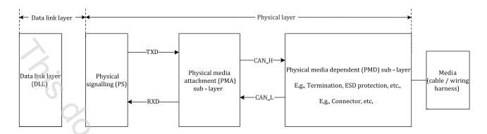
Figure 2 — Implementation example of lower-layers block diagram
