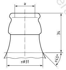
a Ø between 18,0 mm max. and 16,5 mm min. measured at 3 mm max. down from the top, see key d in Figures 4 and 5. Minimum through Ø bore 15,5 mm.
