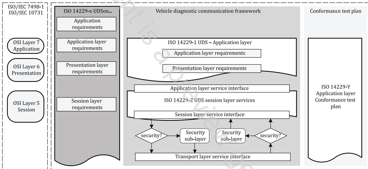
**Figure 1 — ISO 14229 series reference according to OSI model**
