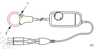
Type A current sensor with fork-style JAWS
