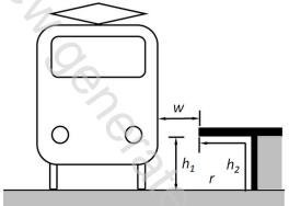
f) Train passing close to a platform at the station envelope,  $e = w + h_1 + h_2$
