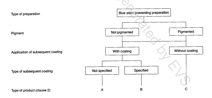
Figure 1: Designation of different types of preparation for preventing blue stain in service
