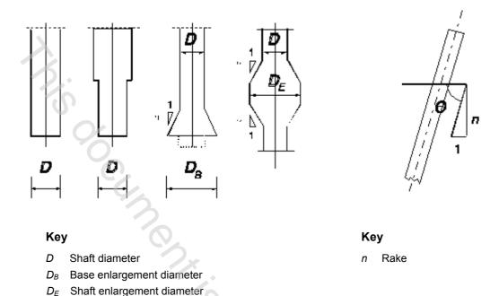
Figure 3 — Examples for straight shaft piles and piles with shaft Figure 4 — Definition of the rake and base enlargement
