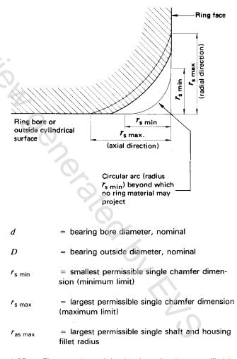
NOTE — The exact shape of the chamfer surface is not specified, but its contour in an axial plane shall not be allowed to project beyond the imaginary circular arc, of radius  $r_{\rm s\ min}$ , tangential to the ring face and the bore or outside cylindrical surface of the ring (see figure).
