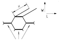
NOTE A set of cells makes up the alveolar material
