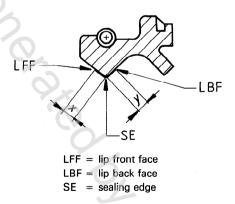
NOTE — Dimensions x and y were chosen because, in case of wear, imperfections in this area impair the function of the rotary shaft lip type seal during its lifetime.
