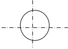
Figure 1. Non-master centerlines incorrectly positioned
