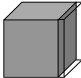
Figure 2. Non-master wireframe structure inconsistent with solid
